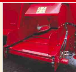
Model VL(K)-T has a chain conveyor with side-shift at front.
