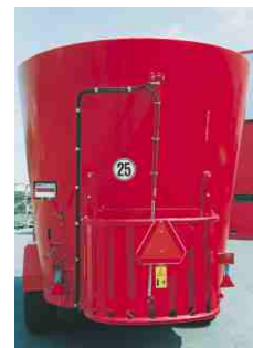
A discharge door at the back of the machine as an option.
