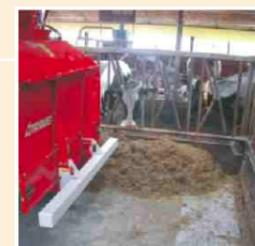
Cross conveyor belt at the back of the machine.
