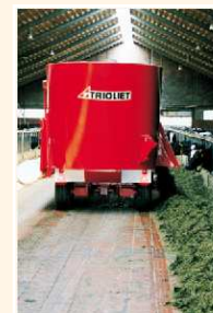
Discharge side doors deposits the feed to the left or to the right, quickly and without spilling.
