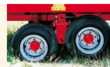
Types ZKT is standard equipped with four single wheels on reciprocating tandemset.
